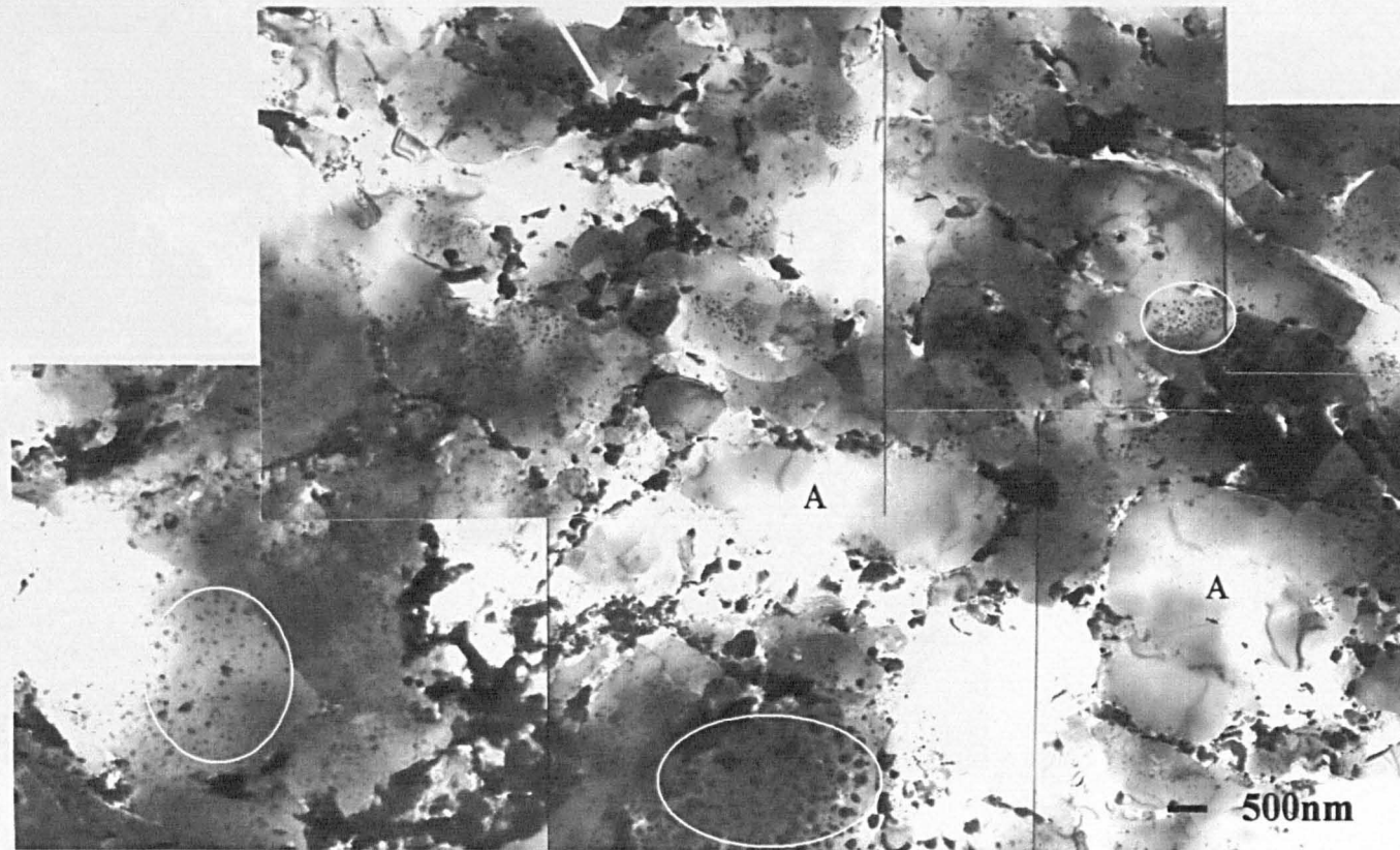
Figure 7.17 TEM montage of the Al 20 Sn 3 Si coating annealed at 300°C for 1 hour.
