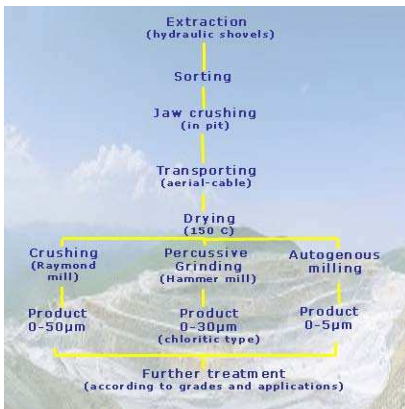
Figure 78: Processing steps followed for talc in Trimouns mines.
