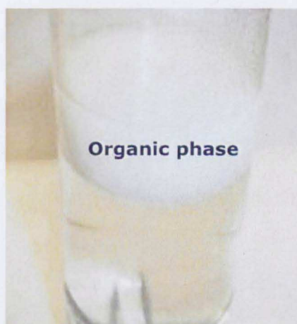
Fig. 7.3: DDSA-HA extraction to the organic layer
