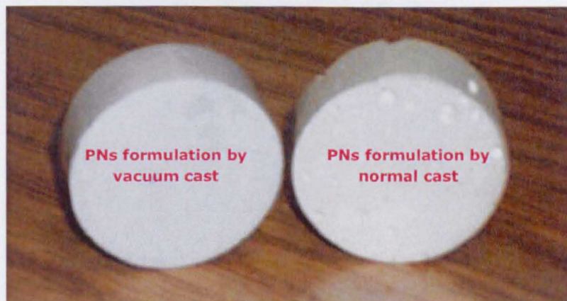
Fig. 4.3: The impact of vacuum cast onto epoxy nanocomposite structural integrity
