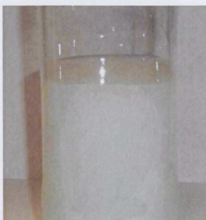
Fig. 6.19: Titania colloid, stabilized via post-synthesis electrostatic stabilization using ammonim phosphate ions
