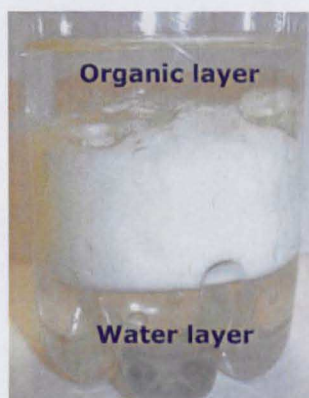
Fig. 5.30: Extraction of TBP-titania using post-modification process
