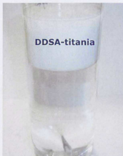
Fig. 5.23: Extraction of DDSA-titania to the organic layer when coating was conducted directly in the reactor using the TIPO precursor
