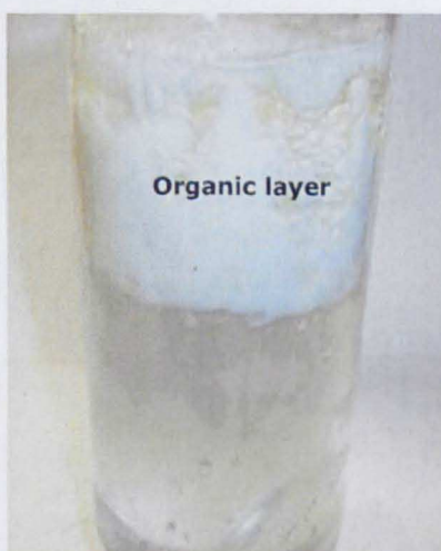
Fig. 6.10: Extraction of poly(ethylene-co-AA 5 wt %)-titania to the organic phase
