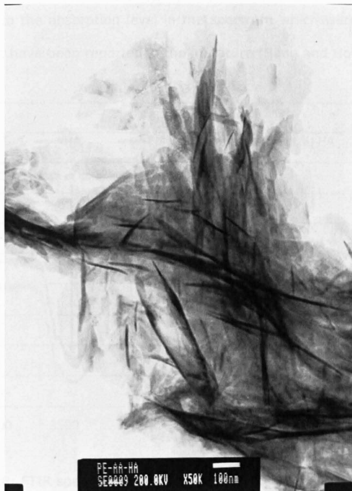
Fig. 7.7: TEM image of poly(ethylene-co-AA 15 wt %)-HA
