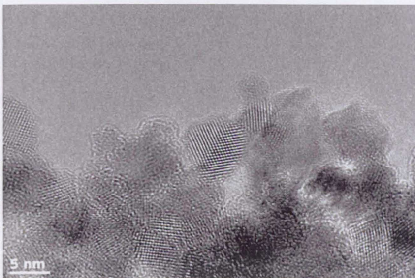
Fig. 5.27: TEM image of DDSA-titania produced via TIBALD modification directly within the reactor using water:IPA mixed solvent system
