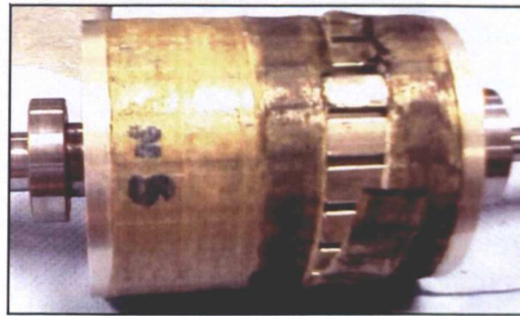
Figure 5-9: The PMSM's rotor and the damaged sleeve
