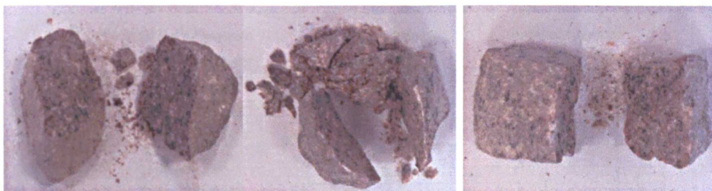
Figure 5.6 Photographs showing the typical daughter fragments produced following the failure of the single parent particles subjected to a diametrical compression test
