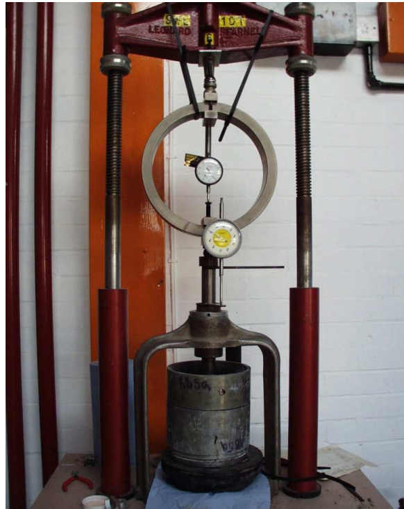
Figure 15: A 7 day swell test sample undergoing CBR testing
