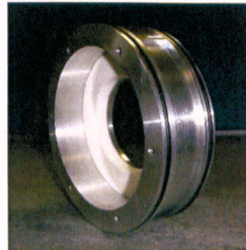
d) Stator housing with water channel
