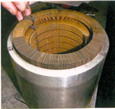
c) Stator housing with laminations
