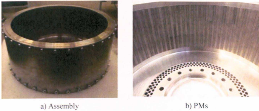
Figure 5.24 GT motor: final rotor assembly
