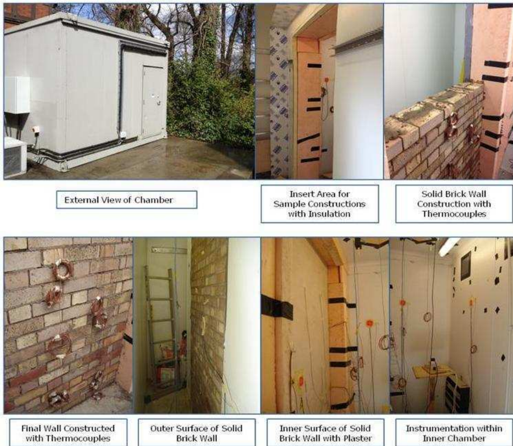
Figure 7-10 - External and Internal Images of Thermal Chamber
