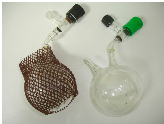
Figure 7.2: Two identical glass vessels used for xenon samples in MRI scanner. Left: thermal sample, right: hyperpolarised sample container.
