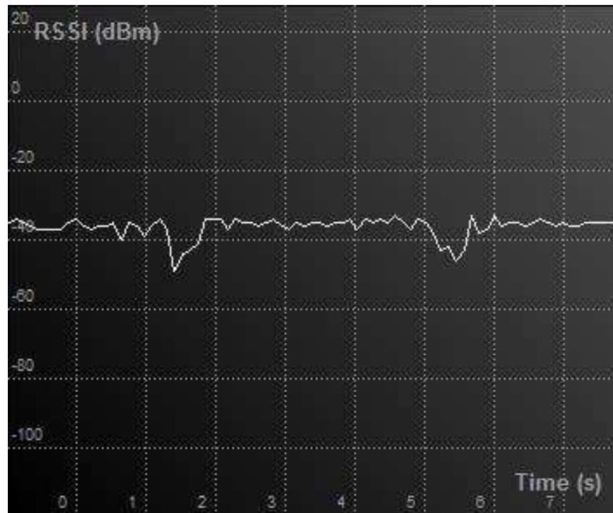
FIGURE 6-6: CHANNEL 100 WITH A 0 dBm SIGNAL AND A PERSON CROSSING THE LOS TWICE
