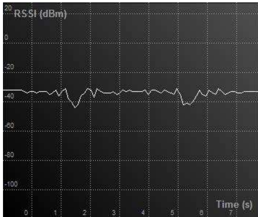
FIGURE 6-5: CHANNEL 50 WITH A 0 DBM SIGNAL AND A PERSON CROSSING THE LOS TWICE
