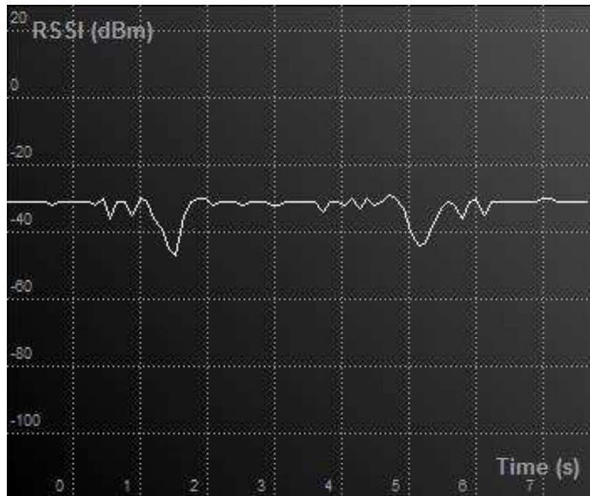
FIGURE 6-4: CHANNEL 0 WITH A 0 DBM SIGNAL AND A PERSON CROSSING THE LOS TWICE
