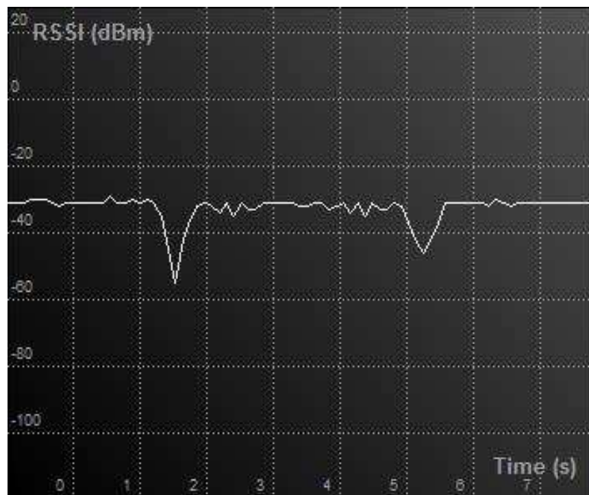
FIGURE 6-7: CHANNEL 255 WITH A 0 dBm SIGNAL AND A PERSON CROSSING THE LOS TWICE
