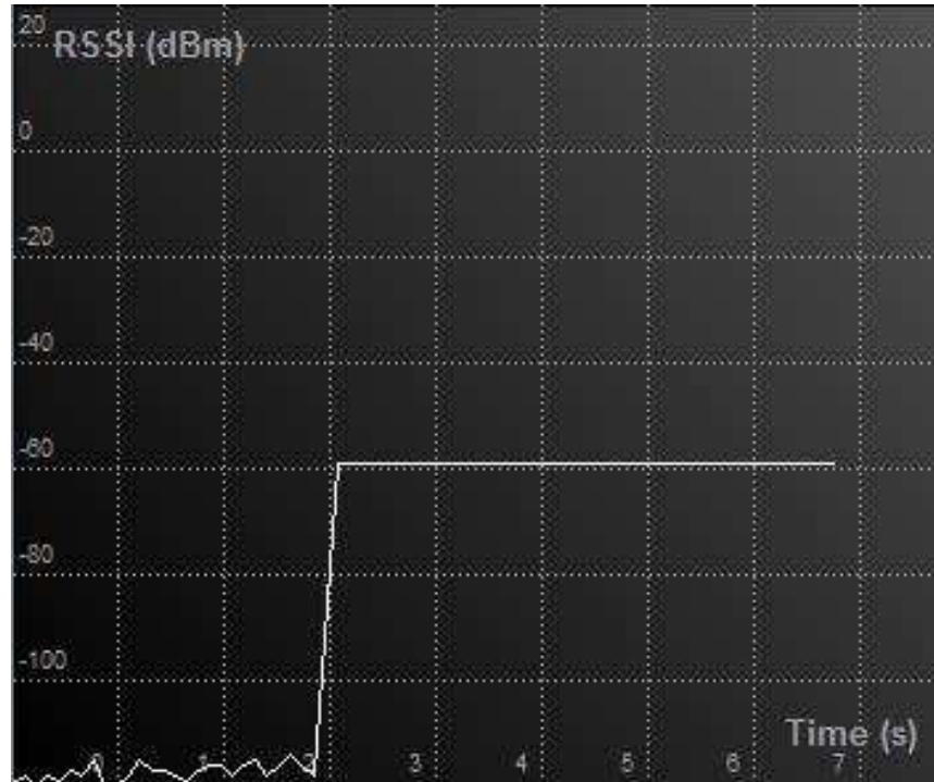
FIGURE 6-10: CHANNEL 0 WITHOUT AND WITH A -30 dBm INPUT SIGNAL
