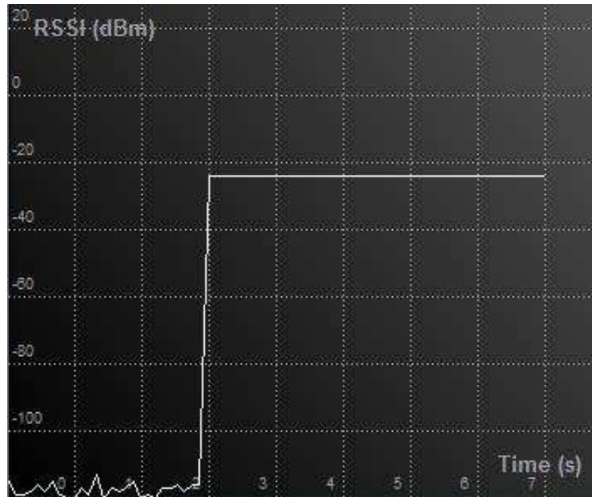
FIGURE 6-8: CHANNEL 0 WITHOUT AND WITH A 12 DBM INPUT SIGNAL
