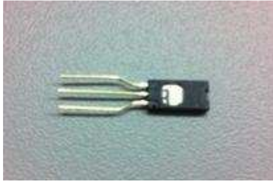
Figure 5-5 Photo of humidity sensor
