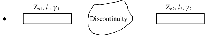
Fig. 2.15 Cascade representation of transmission line with discontinuity
