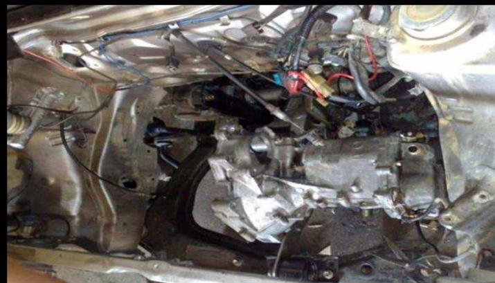
(c) The engine bay void of the engine block and most of the other parts
