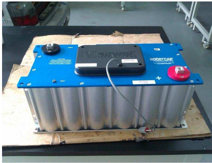
Fig. 46: BMOD0165P048; 165F, 48.6V supercapacitor which weighs 15kg
