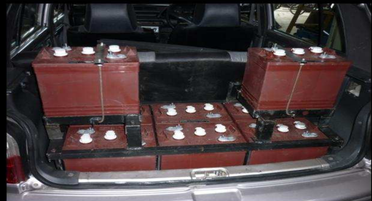
(d) Custom battery racks fitted to the rear compartment of the vehicle
