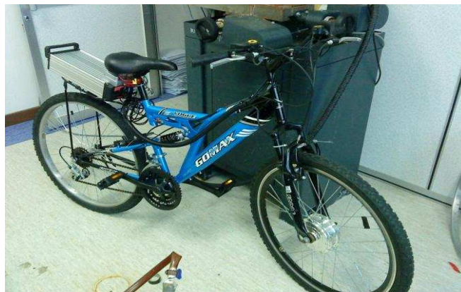
Figure 5: Ebike with battery supercapacitor hybrid via a boost converter.
