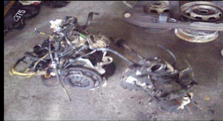
(b) 660 cc Engine block and fuel tank taken out
