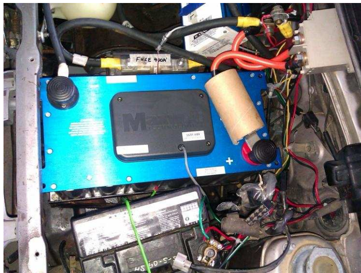
Fig 47: BMOD0165P048 installed just above the electric motor. Top right is the high current contactor which is activated by a 12V coil and a manual switch on the dashboard of the vehicle.
