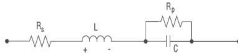
Fig 8: 1 st Order Model of the Supercapacitor
