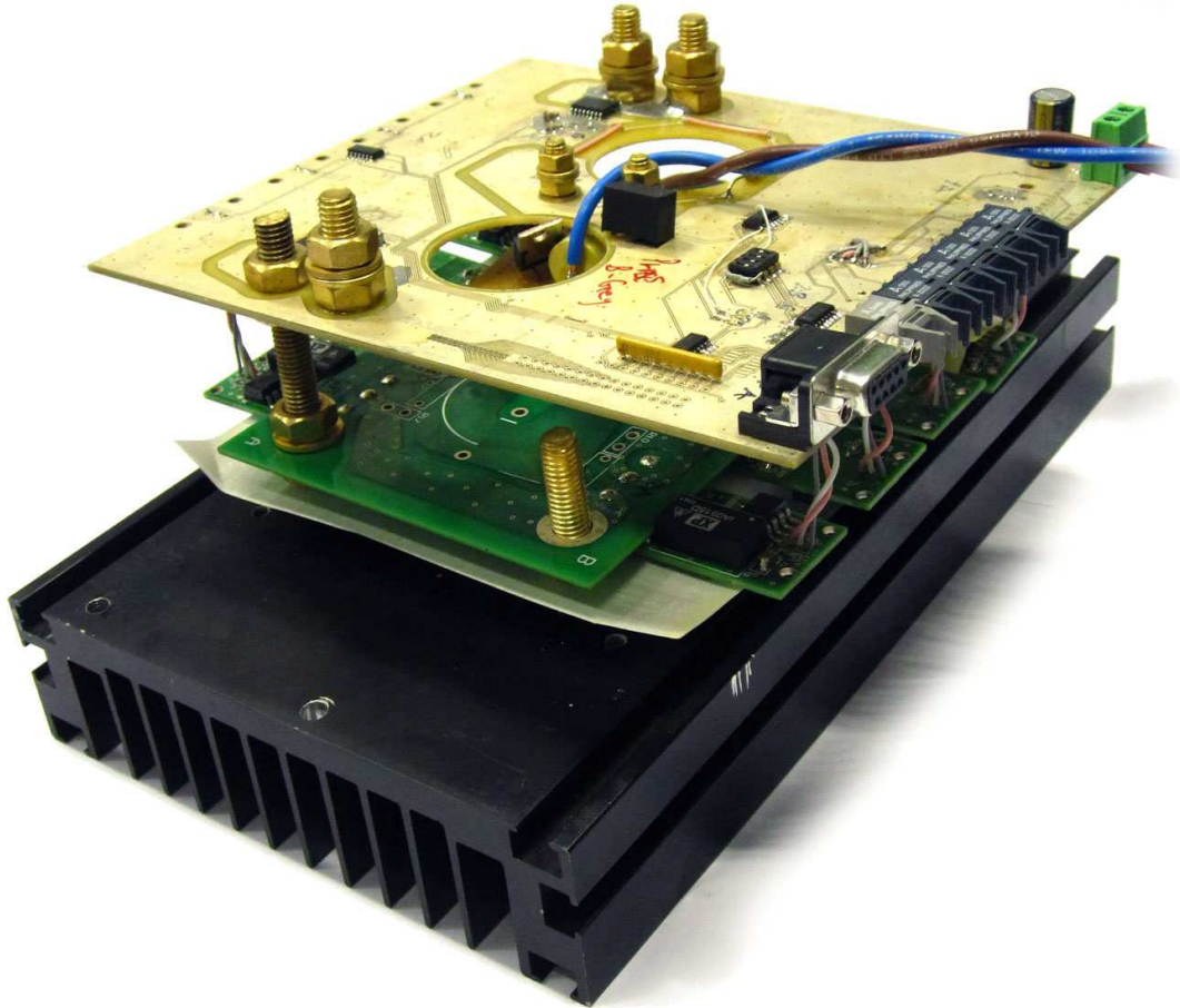
Figure 5.4: Assembled Cycloconverter, with Power, Gate Drive and Control PCBs visible
