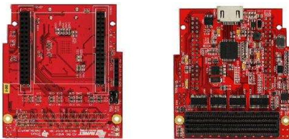
Figure E-1: The left image shows the top of the Avnet FMC module. The right image is for the bottom.
