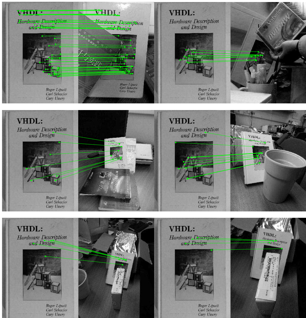
Figure 6-12: Object recognition for planar objects in presence of transformations, cluttered background and partial occlusion.
