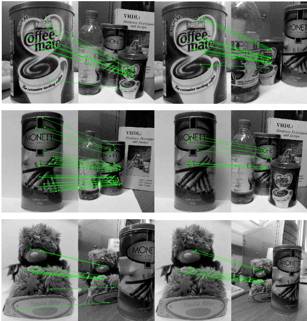
Figure 6-13: Object recognition for 3D objects in presence of transformations, cluttered background and partial occlusion.
