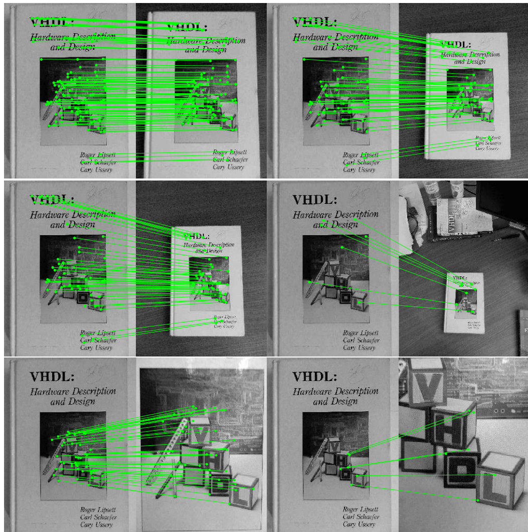
Figure 6-5: Testing results for scale changes. The scaling factors are 0.9, 0.7, 0.6, 0.3, 2 and 3.5, respectively, starting from the upper-left corner.
