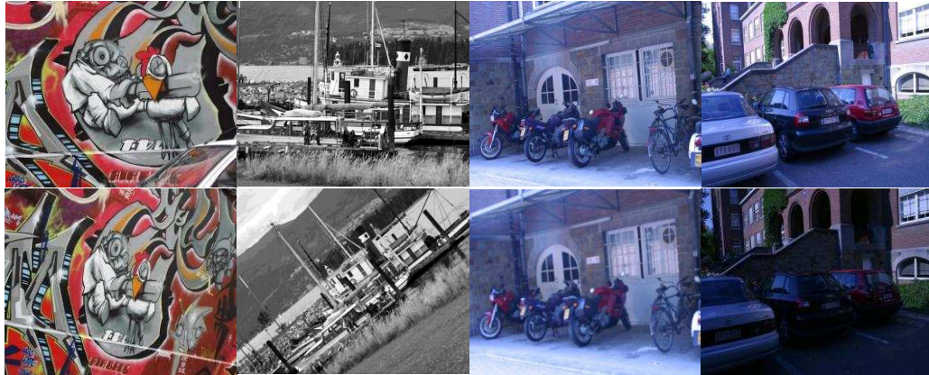
(a) Example images. The first row shows reference images. The second row shows the transformed images. From left to right: graf (viewpoint), boat (scaling+rotation), bike (blur), and light changes.
