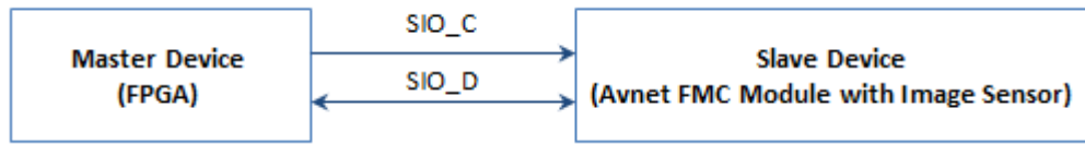
Figure E-2: Function block diagram for the 2-wire SCCB.
