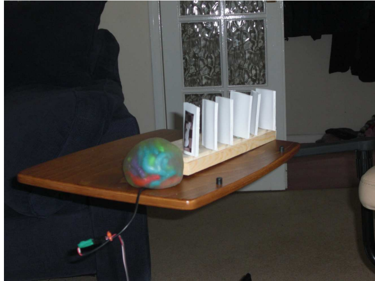
Figure 6.12: Solomon - Prototype device. Pressure sensors are embedded into white cardboard objects. Artefact has been placed on the swinging table that is attached to Solomons chair.
