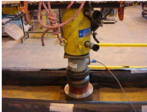
Figure 3.11 Concentrated load jacking system
