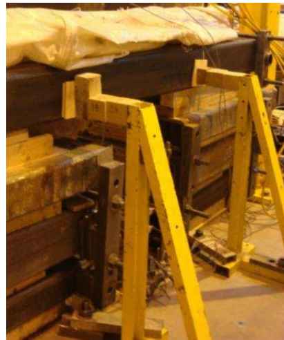
Figure 3.8 Wood wedges on the long beams against 'A' frames
