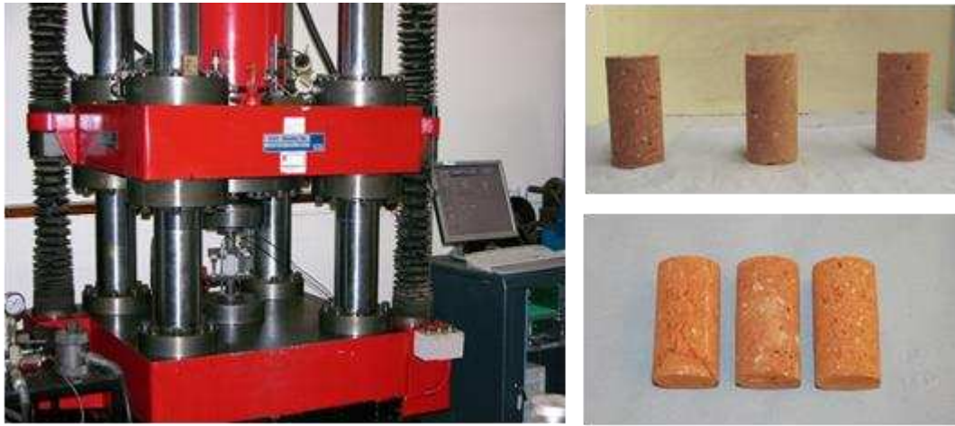
Figure 4.1 (a) Stiff testing machine in NCG; (b) & (c) Brick samples
