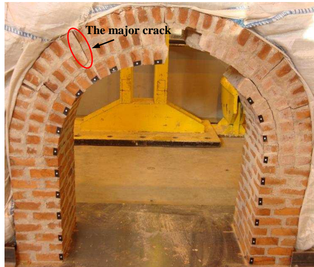
Figure 3.41 The major crack at one third of the tunnel arch of the physical model 3 for the measurement of crack length and width
