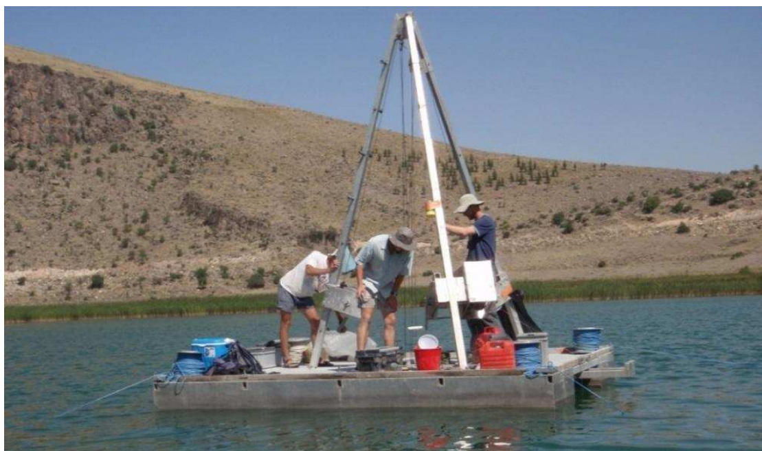
Figure 6.3 UWITEC coring system on Nar Gölü in July 2010.
