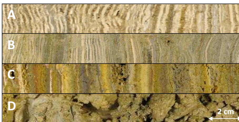
Figure 8.1 Photographs of cores after opening showing different lithologies found in the sequence. A and B show the mm-thick laminations. C shows the cm-thick bands and D the hard, concretioned non-laminated sediments.
