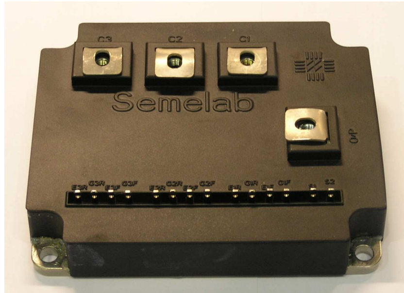
Figure 5.6: Photograph of the power module
