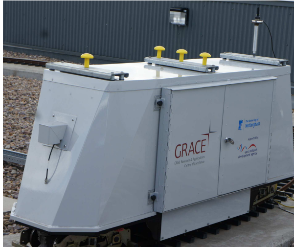
Figure 5.3 – Mounting of Locata antenna on a train during the kinematic trials
