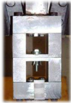
Figure 2.7 Set-up for direct tension tests on Holo-bolts (Elghazouli et al. 2009)
