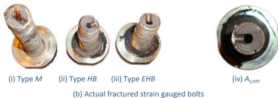
Figure 5.14 Net tensile stress area
