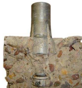
(c) Breakout forming at approx. 20^\circ
