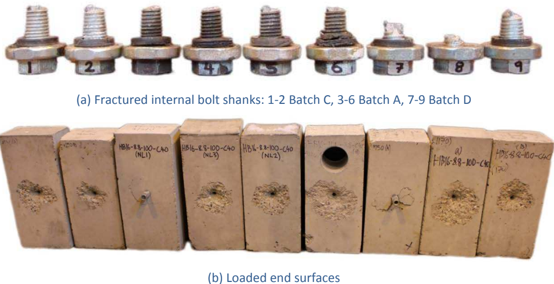
Figure 5.26 Benchmark specimen failure mode (HB16-100-8.8-C40)
