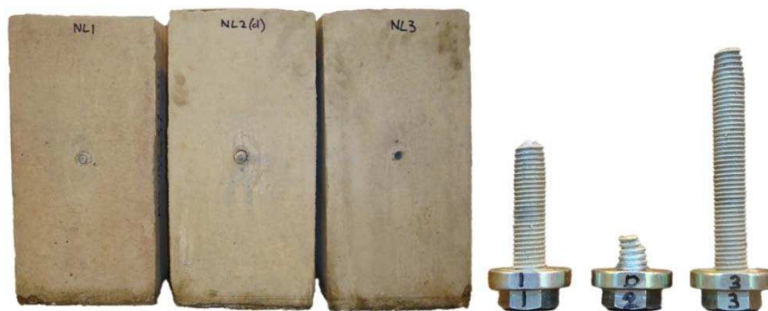
Specimens M16-150-8.8D-C40-1, M16-150-8.8D-C40-2, M16-150-8.8D-C40-3 (left to right)
