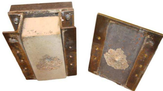
(a) loaded end surface of pull-out specimen after testing
