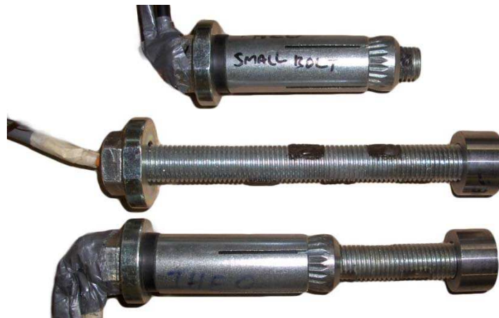
Figure 4.8 Instrumented bolts: fully assembled ready for tightening / testing
