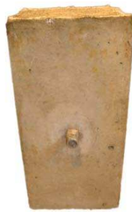
Figure 5.29 Effect of high strength concrete on failure mode (in HB16-100-8.8D-C60-1)
