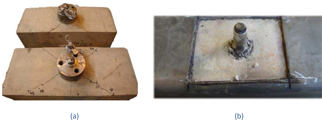
Figure 3.21 Specimens after testing (a) unconfined, (b) confined
