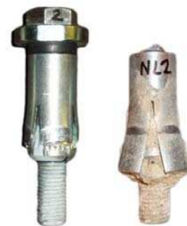
(c) effect of concrete on expanding sleeves
