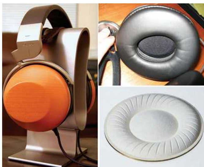
Figure 2.15: Nanocellulose diaphragm used in SONY headphones [116].
