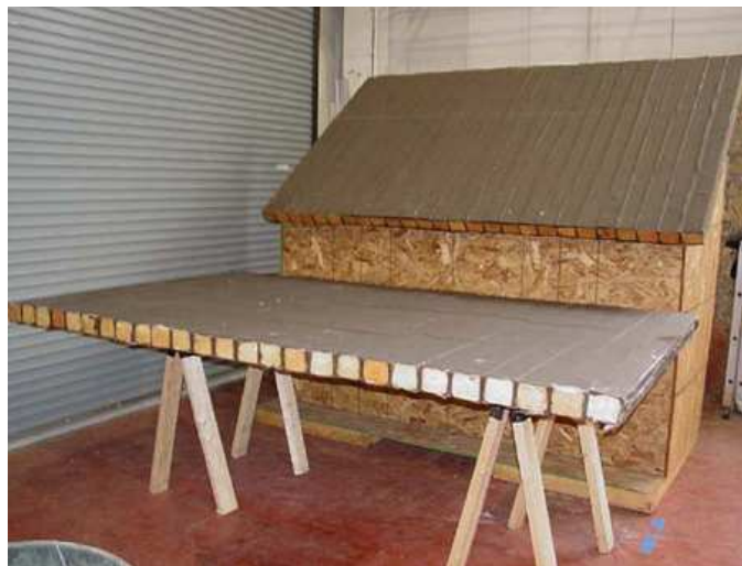
Figure 2.9: Roof panel prepared using biocomposite materials [118].
