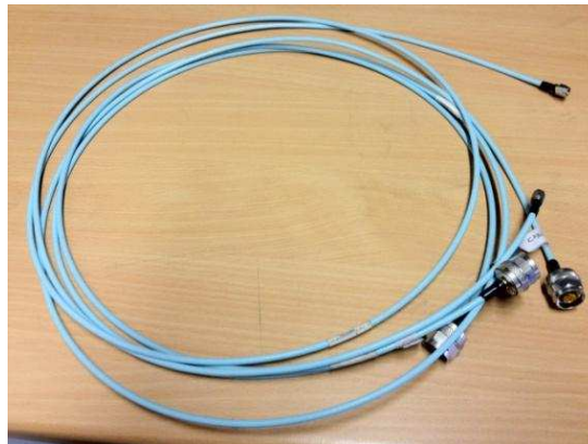
Figure 3.1.1: Typical SMA/BNC cables used to provide connections
