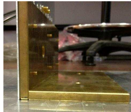
Figure 3.2.9: The arrangement of two RG-58 coaxial cables above an aluminium ground plane. (a) Side view. (b) Plan view. (c) Back view. (d) Brass end plate placed on the aluminium ground plane.
