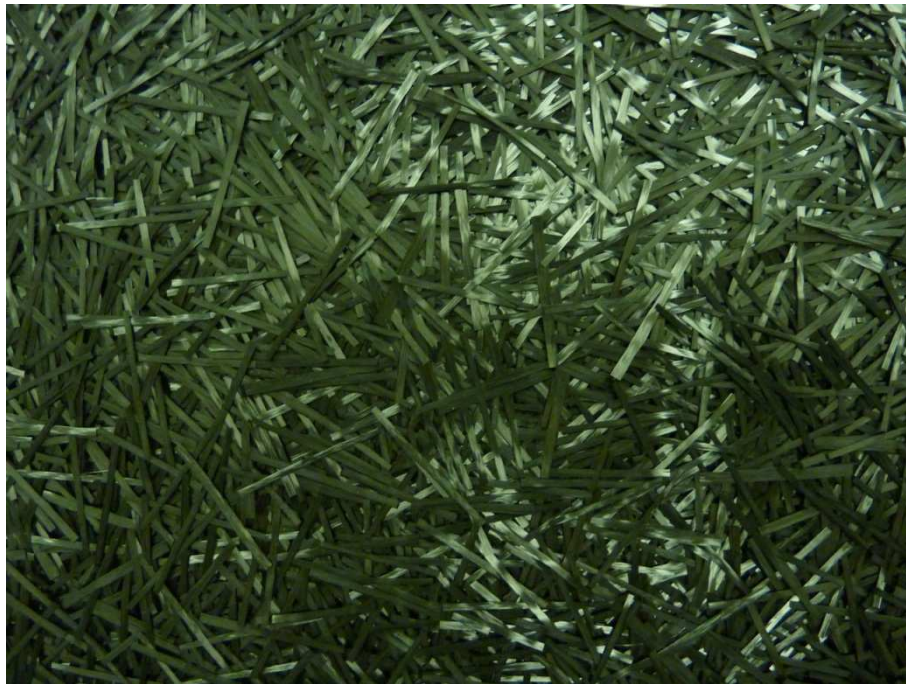
Figure 34: FA2 preform incorporating a distribution of 3k, 30 mm tows.
