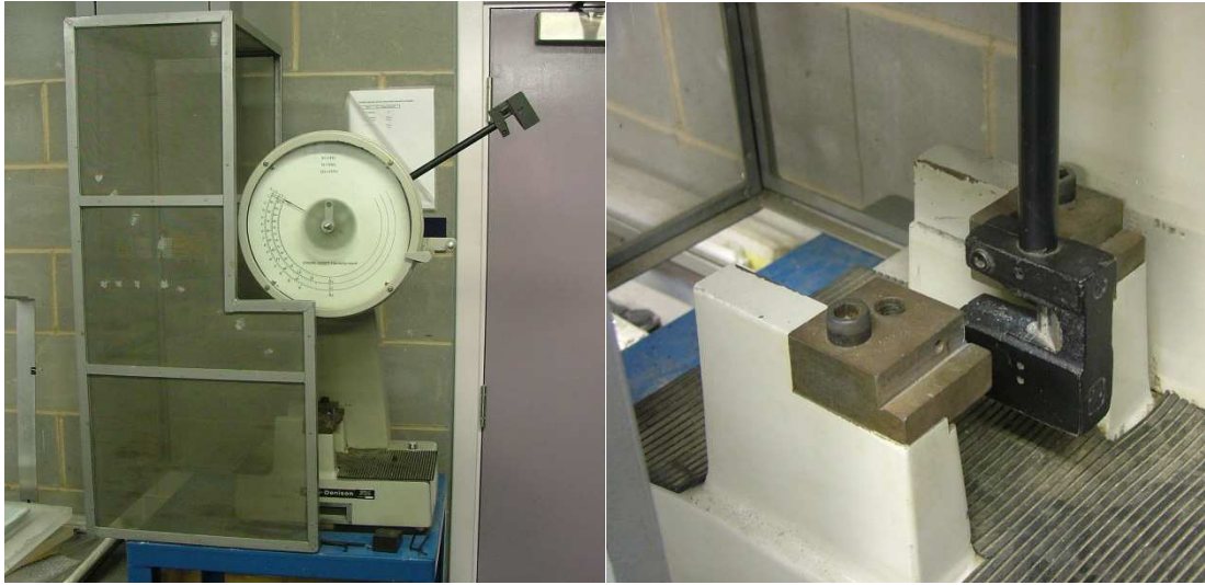
Figure 13. Avery Denison Charpy impact test machine.
