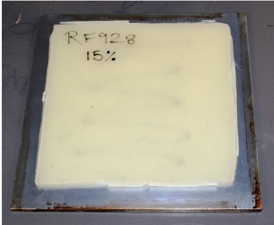
Figure 62. Neat resin sample produced from a blend of Prime 20LV and 15 phr Hypox RF928. The formulation remained clear before moulding, but phase separation of the CTBN rubber occurred during cure to produce a distinctly cloudy appearance in the moulded sample.
