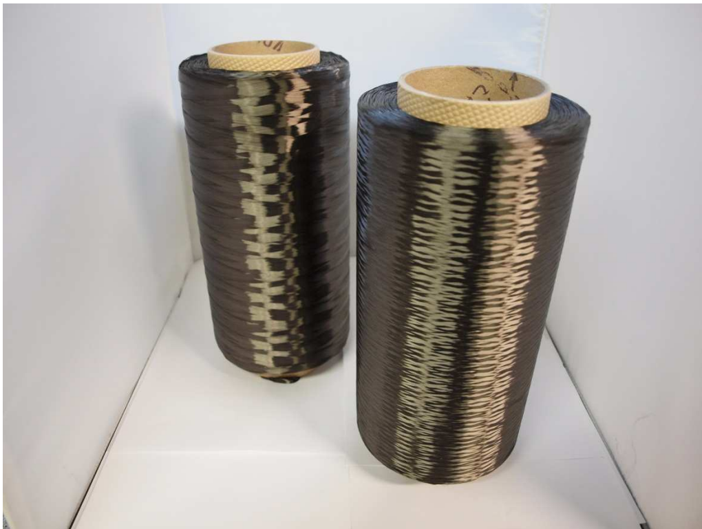
Figure 3. Carbon fibre tows, containing several thousand filaments of carbon (left – 24k, right – 3k), wound around bobbins.
