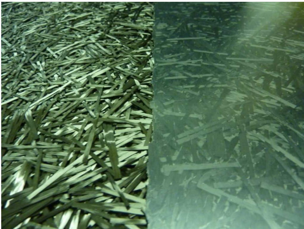
Figure 78. 3k, 30 mm (FA2) DCFP fibre architecture. The preform is shown on the left and the “A-side” of a moulded part is shown on the right.
