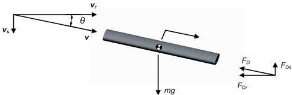
Figure 4-18: Free body diagram of the forces and velocity components acting on a tow segment during flight in the plane of motion.
