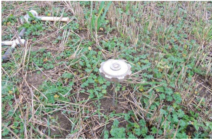
Fig. A.1. Estimation of shear strength in the field using hand held shear vane
