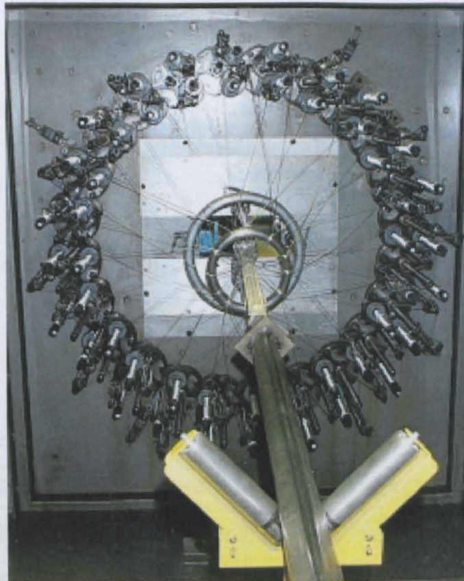
Figure 3-6 – The braiding of the 38.1mm diameter small braided tubes
