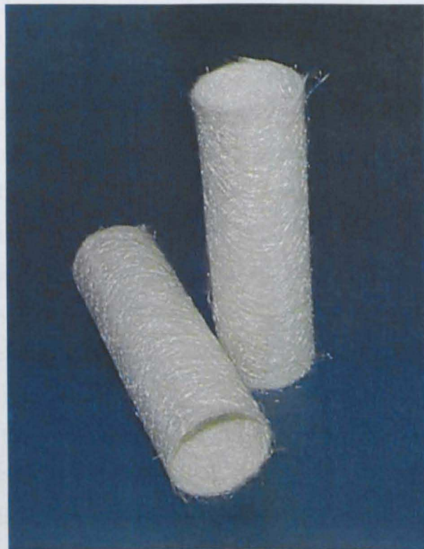
Figure 3-4 – Preforms (from Duckett [5])
