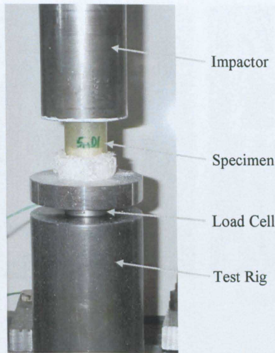
Figure 3-17 – Dynamic tube test rig
