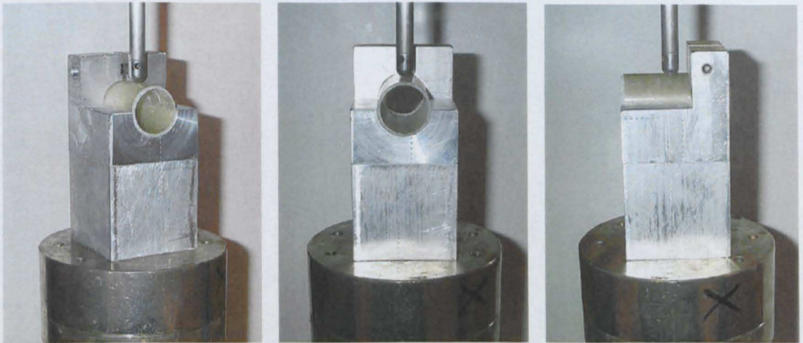
Figure 3-12 – Fixture used to add damage to and drill small (38.1mm diameter) tubes
