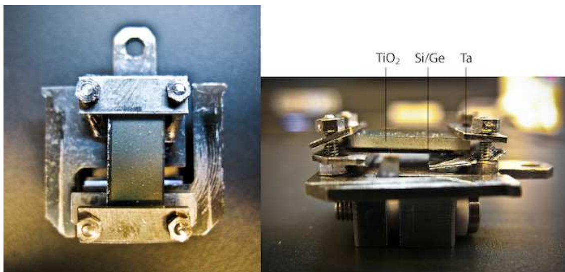
FIGURE 6.2: Photographs showing a TiO 2 substrate clamped using Ta to a Si crystal.
