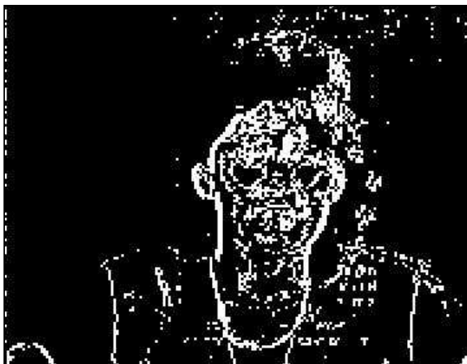
Figure 6.6.3: Location of motion vector origins, Miss America frame 032, \Delta Q=8 , QCIF resolution
