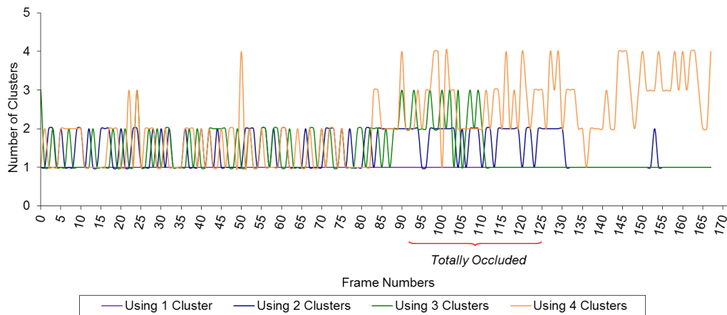
Figure B.2 Graph showing the use of different numbers of clusters for a yellow circle experiencing occlusion amid clutter.
