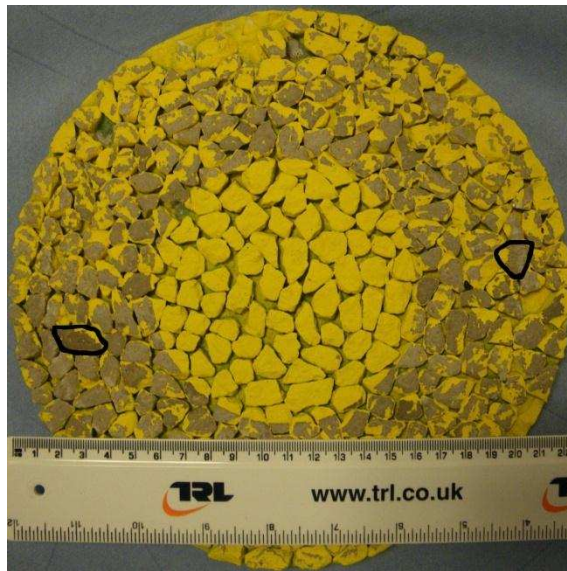
Figure 5.19 Limestone test specimen after painting and polishing
