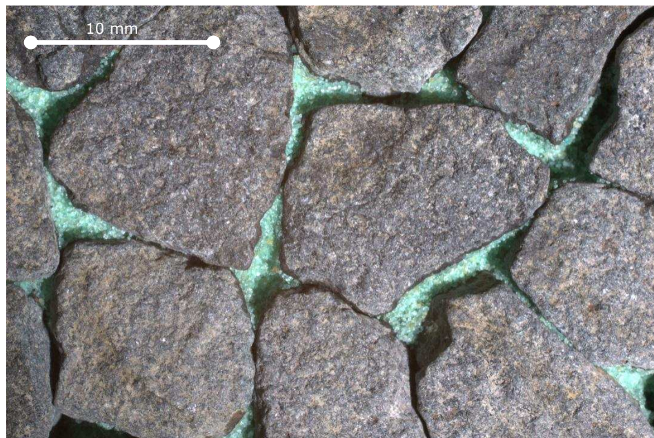
Figure 4.2 Dolerite aggregate specimen prepared for polishing
