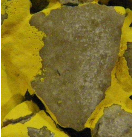
Figure 6.8 Limestone aggregate particle after painting and subsequent polishing
