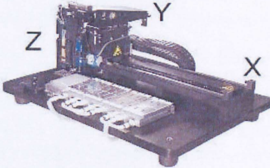
Figure 2.4: Photo of the stage showing translation axes [83].
