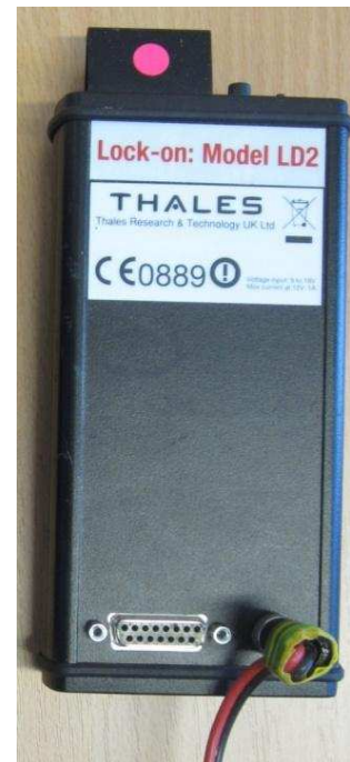
Figure 4.2 UWB unit that can be configured as either base unit, mobile unit or control unit
