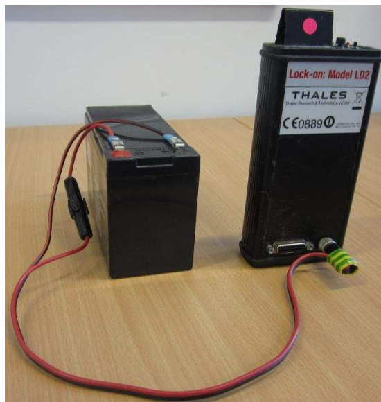
Figure 4.3 UWB mobile unit set up, connected to a 12 Volt battery
