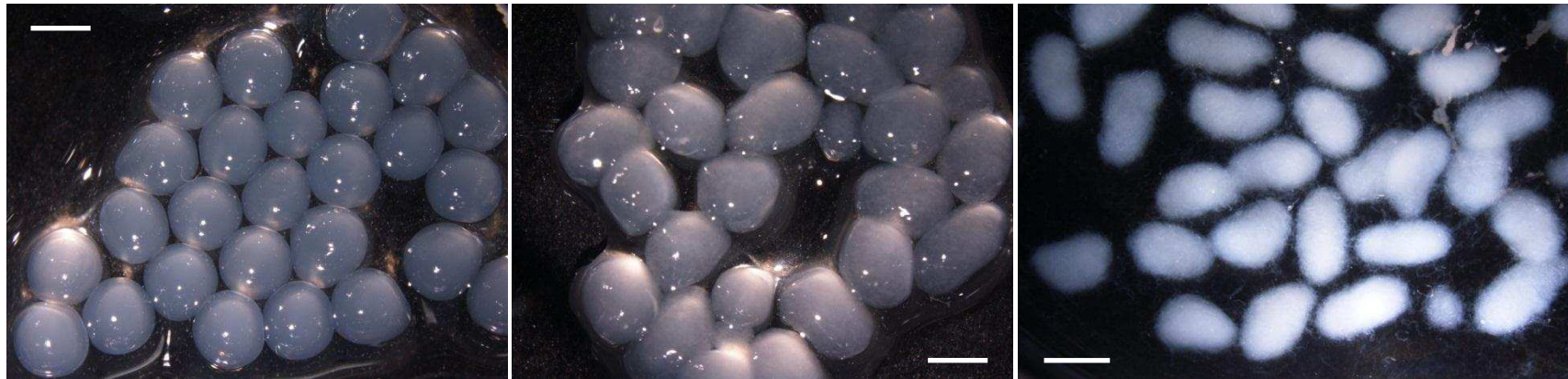
Figure 4.12 – Representative bright field microscopy images of (left to right) – hydrogel beads composed of alginate alone, beads produced from a 2:1 (v:v) ratio of DECM digest to alginate solution and beads produced from the same ratio of DECM to alginate imaged after treatment for 10 minutes with 0.25 M sodium citrate to remove the alginate component. Scale bars represent 2 mm.
