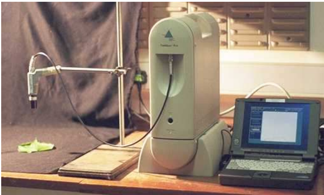
Figure 3.4 ASD Fieldspec Pro showing computer interface and fibre optic probe.
