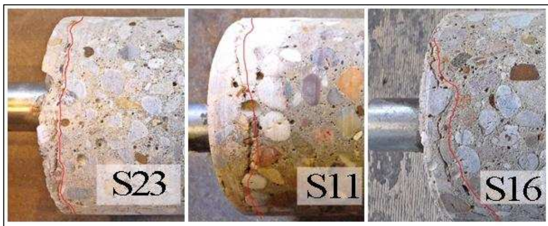
Figure 4.17 : Crack propagation on the concrete at stress ranges 584, 455, and 325 \text{N/mm}^2
