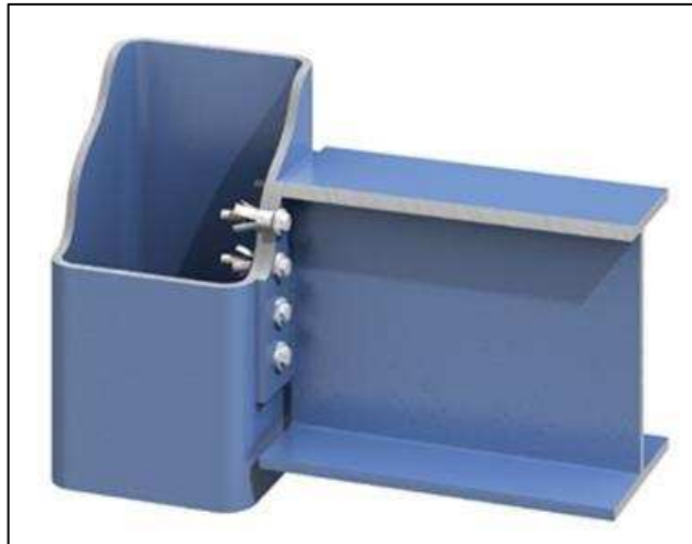
Figure 1.1: Typical endplate connection to a tube (Lindapter, 2012)
