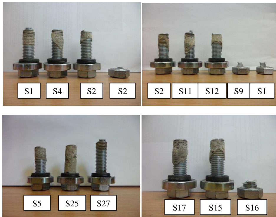
Figure 4.4 : Failure mode of Extended Hollobolt
