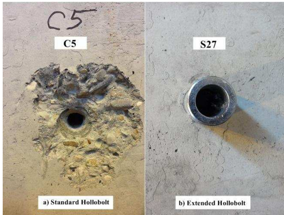
Figure 4.11 : Concrete surface of the standard HB and EHB test specimens
