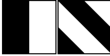
Figure 3.1: Sod shock test initial conditions.
