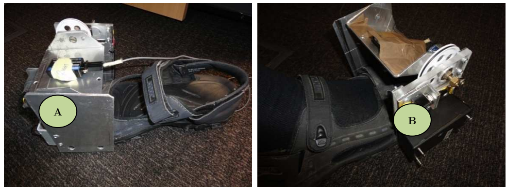
Fig. 7.16: RIMU prototype with (left) IMU mounted on a rotating platform, and (right) the RIMU controller
