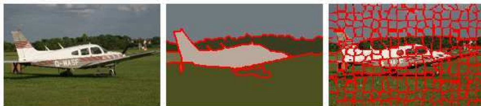
FIGURE 4.6: From left to right: original image; object-like regions generated by our full model; superpixels commonly used in conventional semantic segmentation methods
