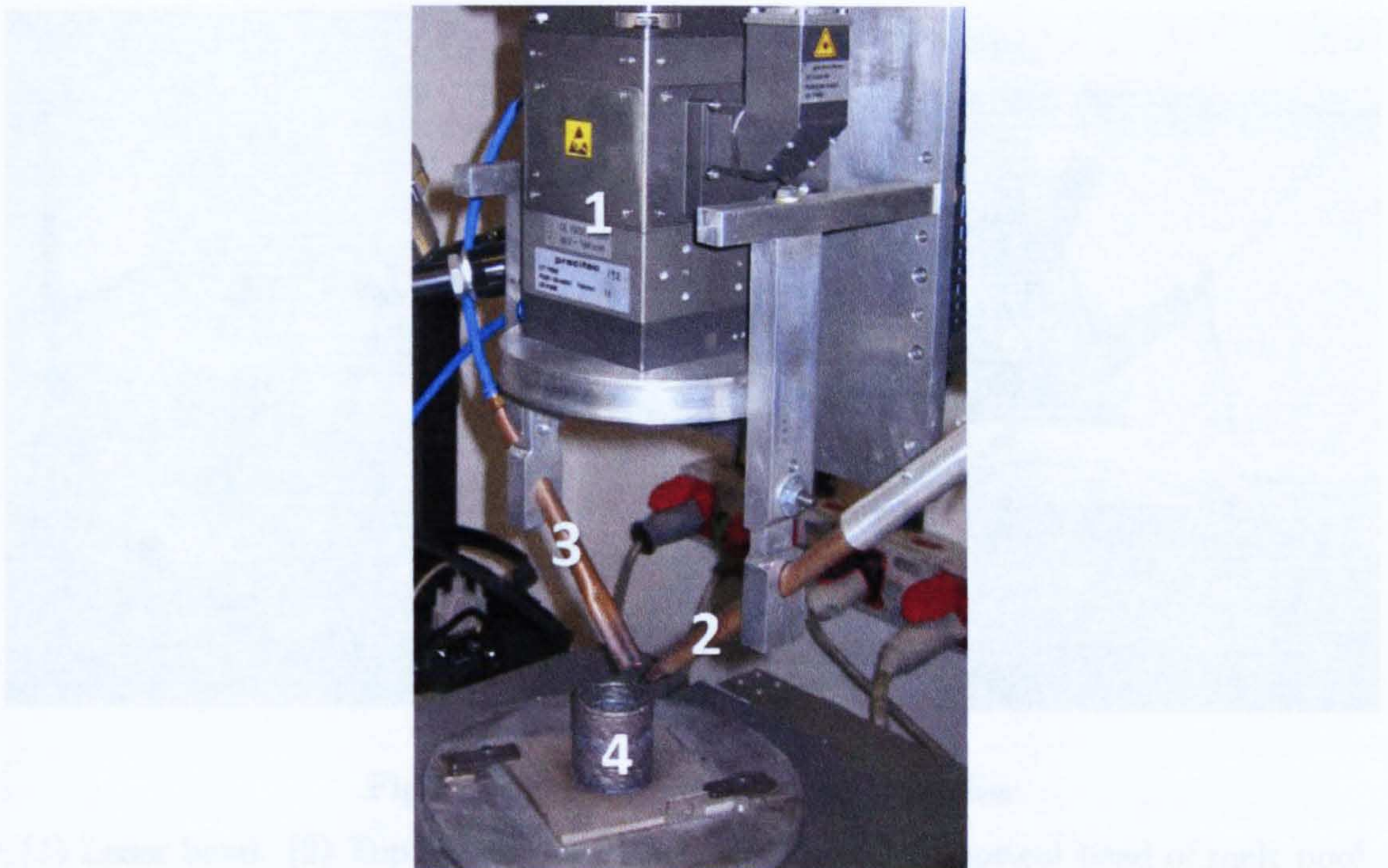
Figure 3.1: Initial setup of the metal deposition system (1) Laser head. (2) Wire feeder nozzle. (3) Argon nozzle. (4) Workpiece (38 mm diameter cylinder).
