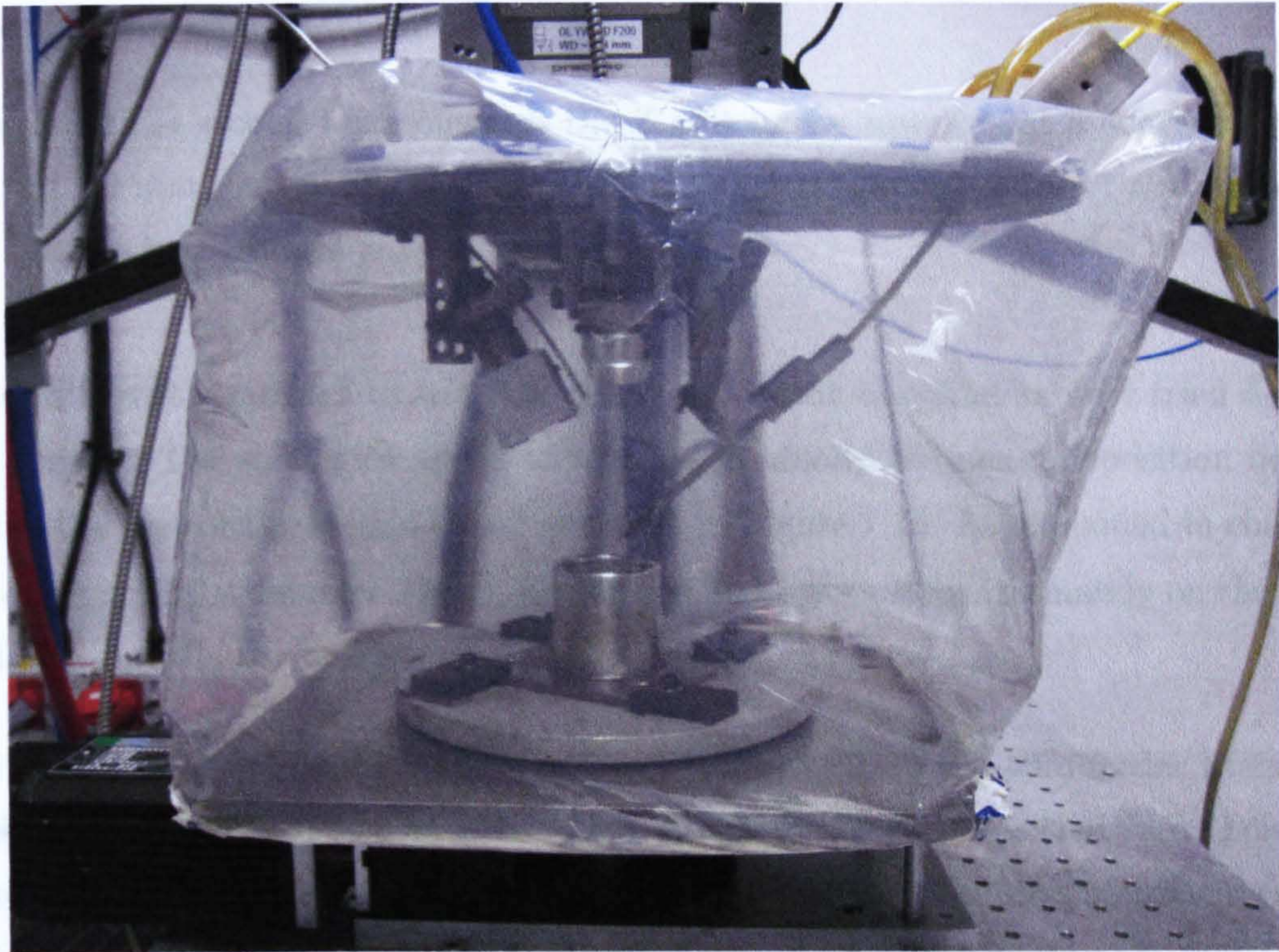
Figure 7.15: Deposition of a cylinder inside argon chamber The diameter of the cylinder is 50 mm.
