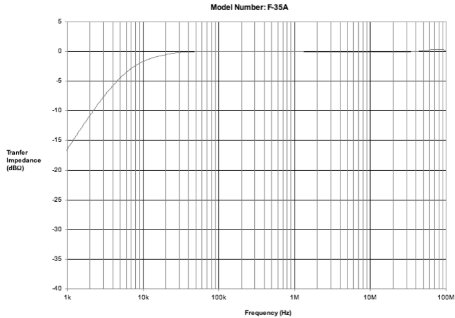
Figure 5.3: Calibration curve for current probe FCC F-35A
