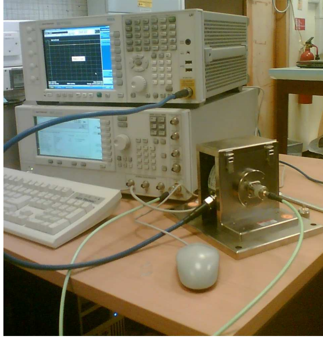
Figure 5.4: Setup for current probe calibration
