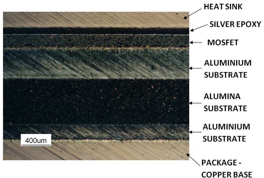
Figure 8.8: A photo of the sectioned MOSFET package with an attached heat sink. The labels show the visible components of the package.
