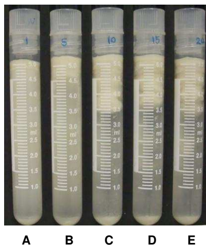
Figure 5.42 Stability test after 24 hours of oil body suspension prepared from hot air stabilized rice bran
