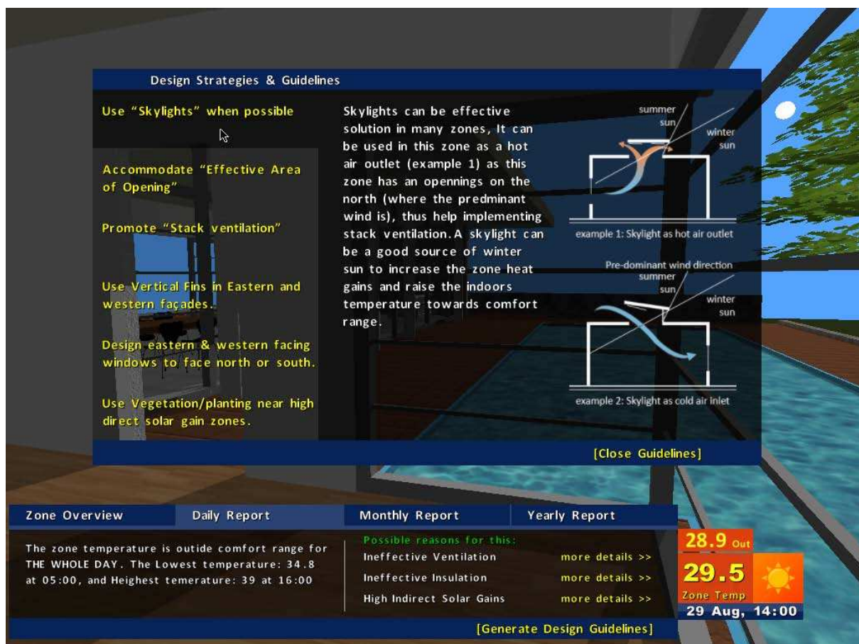
Figure 5.21: Presenting a set of general, building-specific, and zone-specific guidelines in one of the thermal zones, highlighting the benefits of using skylights in this particular zone, along the hot and cold weather conditions.
