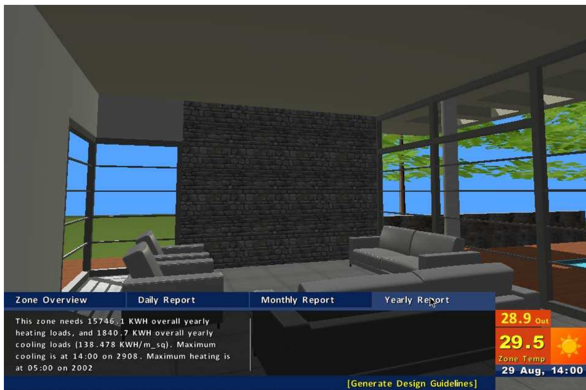
Figure 5.15: Yearly zone report, highlighting the overall required heating and cooling loads for the zone being experienced. The report presents the dates in day-month format (ddmm) and time in hour-minutes format (hh:mm).
