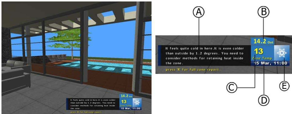
Figure 5.12: The 'Zone Brief' report GUI, representing a brief summary about the current condition of the zone being experienced (A), with presentation of outdoors temperature (B), indoors temperature (C), current date and time (D), and whether the current zone's condition is below, within, or above comfort range temperatures (E).
