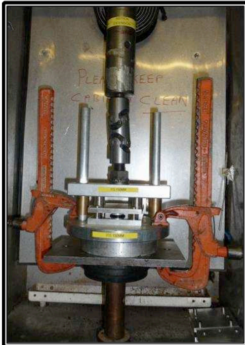
Figure C.8 Test setup (i.e. pair of plates, rigid testing rig and universal joint attachment) is positioned in the INSTRON servo hydraulic frame
