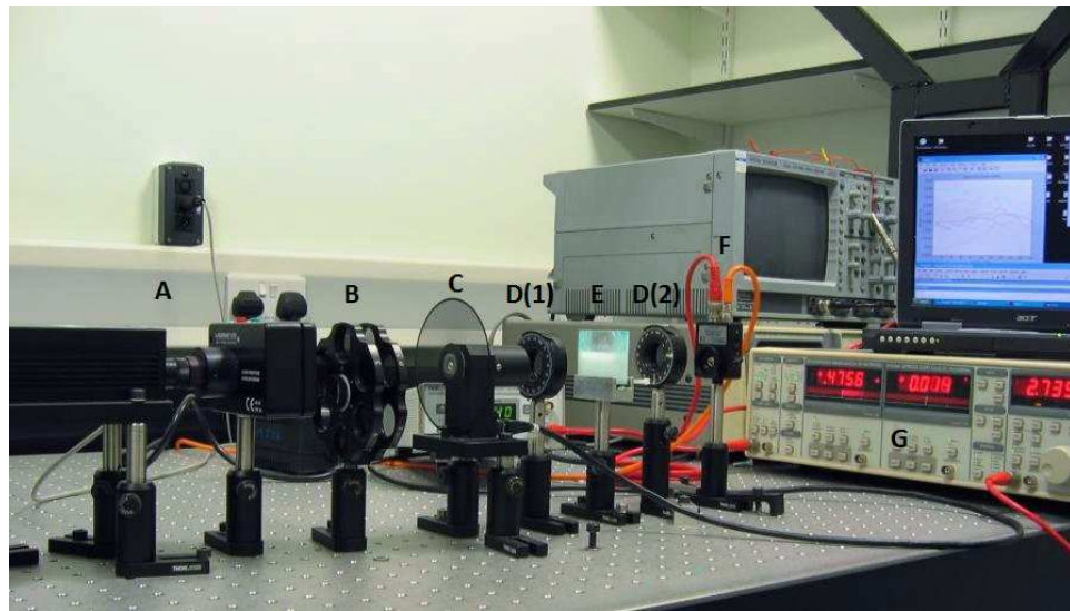
Figure 3.2: The actual polarisation measurement setup. In the diagram- A : laser source, B : optical density filter, C : optical chopper, D(1) : polariser(1), E : sample, D(2) : polariser(2), F : photodetector, G : lock in amplifier. The convex lens used to focus the transmitted light on to the detector is not shown here.
