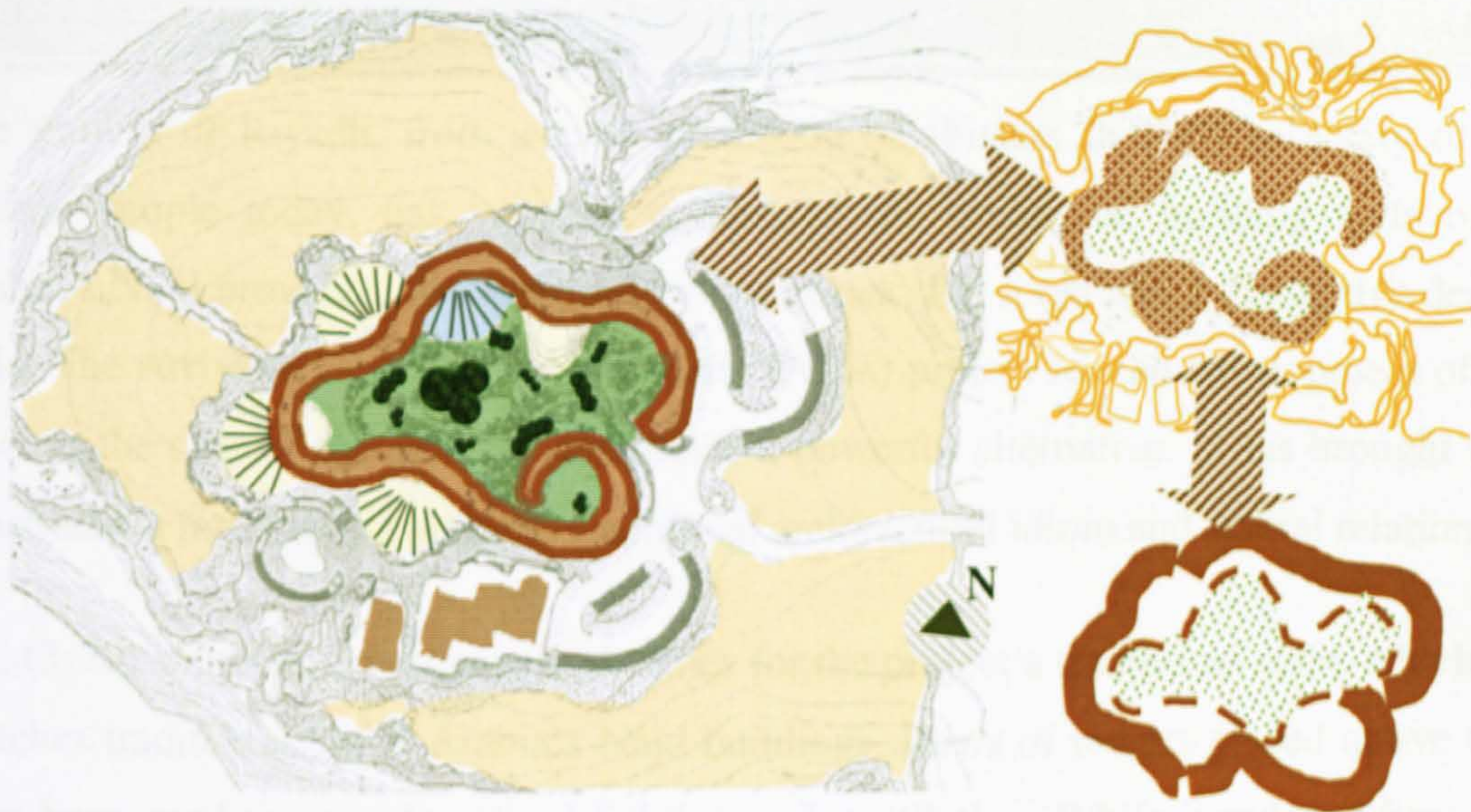
Figure 3-18 The Project Layout Shows the Windowless External Walls and Inner Walls with Small Openings View the Main Courtyard [13]
