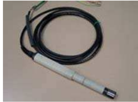
(a) Type K thermocouples (b) Humidity sensor (Vaisala HMP45A)
