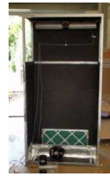
(h) Fans and filter components of cooler
