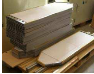
(c) Finished heat/mass exchanger sheets
