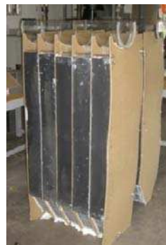
(g) Finished heat/mass exchanger
