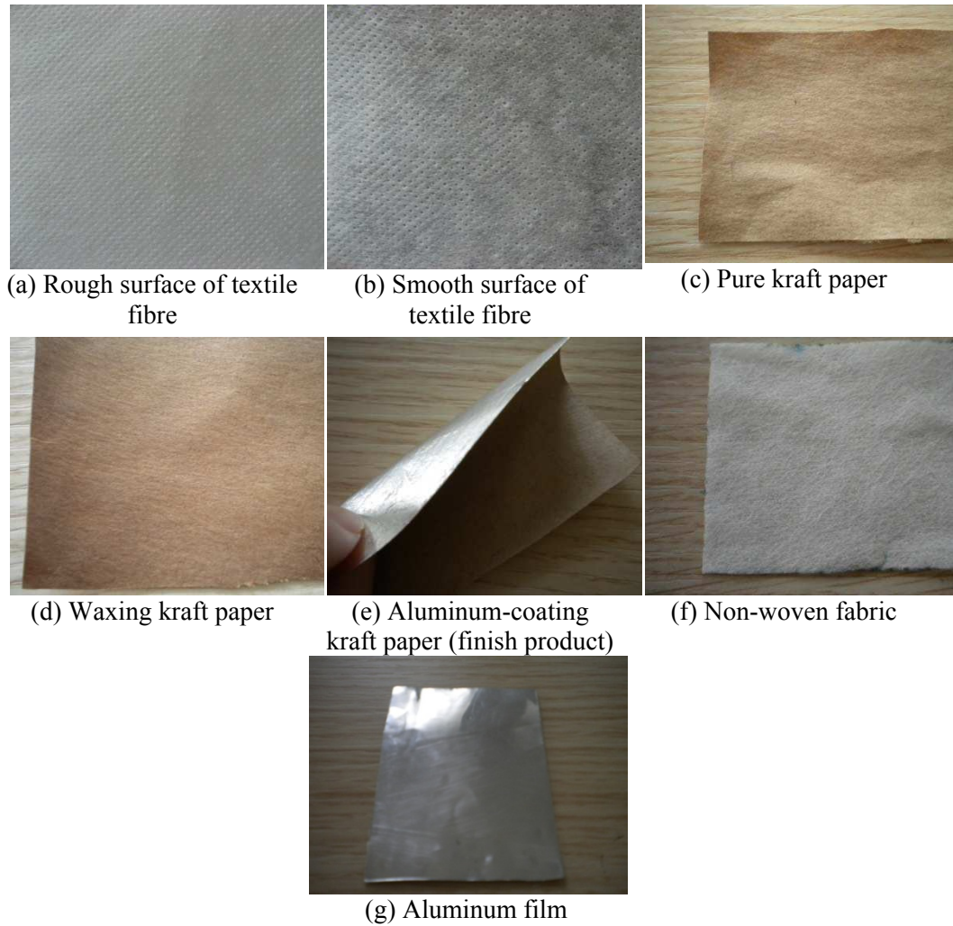
Fig.4-2 The chosen materials for forming heat/mass exchanger
