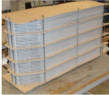
Fig. 5-17 Bolting up of the exchange sheets stack
