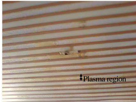
Figure 10.1.1. Detail of burnthrough of electrode sheet after the PEF = 50Hz experiment. Note discoloured regions and pitted areas of the Mylar material in plasma regions.
