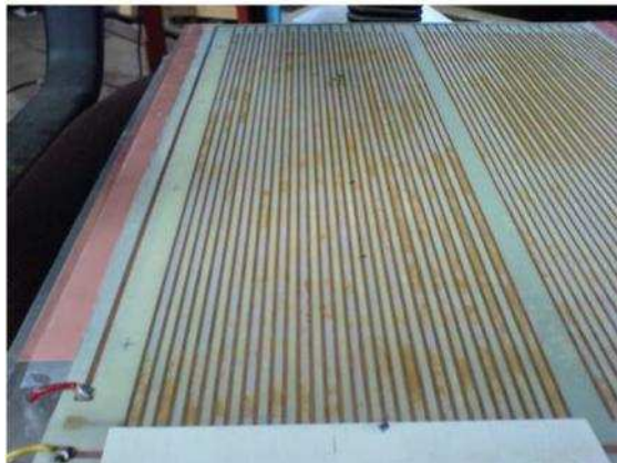
Figure 10.1.1. Detail of burnthrough of electrode sheet after the PEF = 50Hz experiment. Note discoloured regions and pitted areas of the Mylar material in plasma regions.
