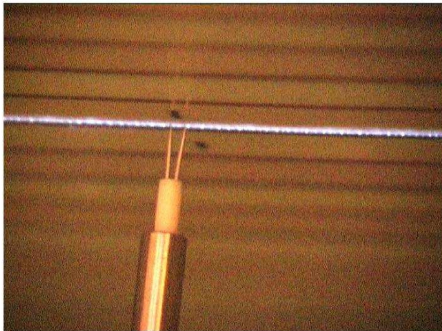
Figure 5.3.11. Colour enhanced images of the asymmetric plasma actuator at: a) t \approx 40\text{ms} ; b) t \approx 80\text{ms} after plasma initiation. Hot wire shown in figure and the prongs have 1.25mm spacing at their tip. The plasma occurs on both sides of the electrode at initiation (a), although the plasma on the near side appears to be brighter and more uniform. After the first few pulses (b), the plasma formation is entirely one-sided.
