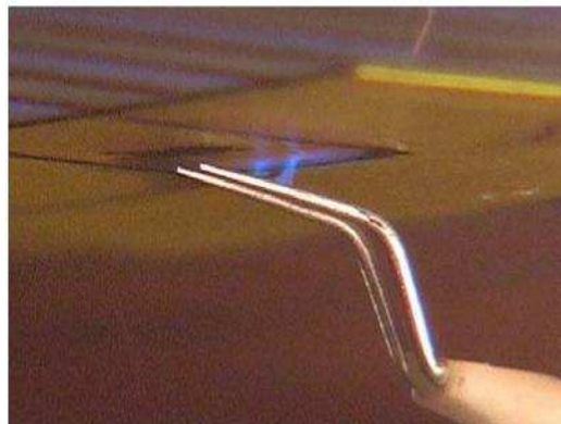
Figure 8.2.5. Insulating tape is used to inhibit plasma formation at the end of the electrodes. However, plasma can be seen to form between the electrode bus (under the tape) and the hot wire, necessitating measurements to be taken an additional 10mm downstream from this position. Remarkably, no damage was caused to the hot wire.
