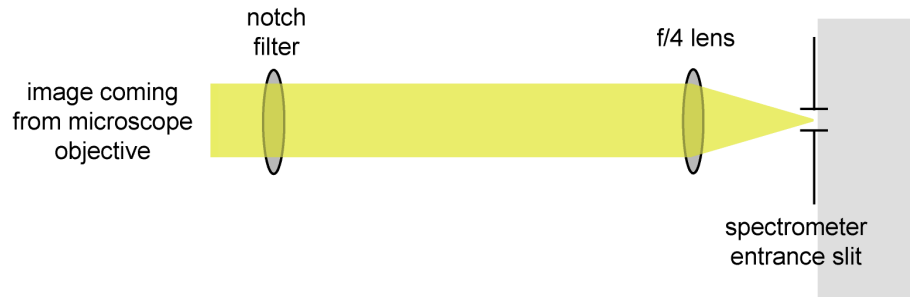
Figure 5.5: Focusing light from the microscope into the spectrometer.
